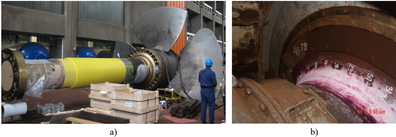
Fig. 1. Disassembled turbine shaft with runner, a) Transition (fillet) zone with cracks b)
