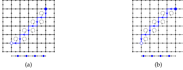
Figure 3.8: Electric string in Q6VM in the AFM phase v < -1 : When v < -1 , the energy is minimized by maximizing the number of flippable plaquettes. Thus, the system displays a ground state described by the maximally kinked string with suppressed quantum fluctuations (in contrast to FIG. 3.7), approaching the diagonal of the bounding rectangle whose opposite vertices are the defects Q = \pm 2 . and the corresponding bosonic picture is a CDW[HAMS19].
