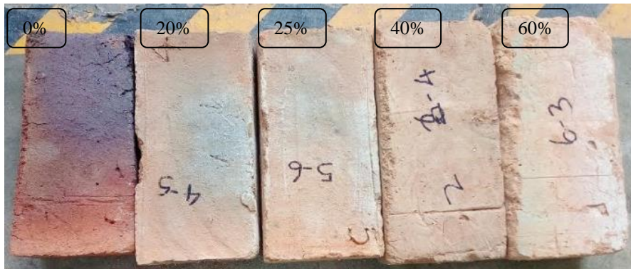
Fig 7 - Burnt bricks with different fly ash contents
