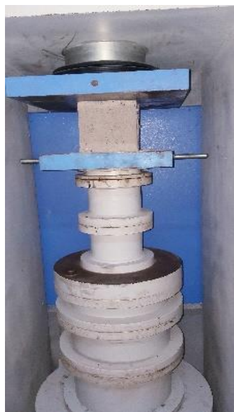
Fig. 1 - Cube compressive strength testing setup
