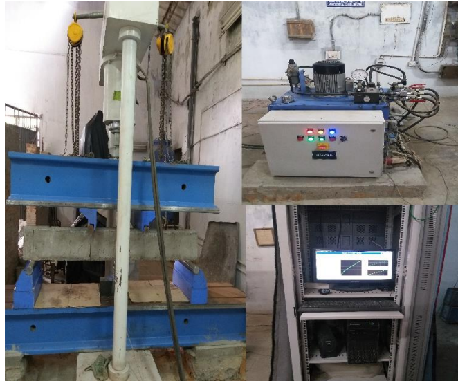
Fig. 2 - Experimental setup of reinforced concrete beam in bending
