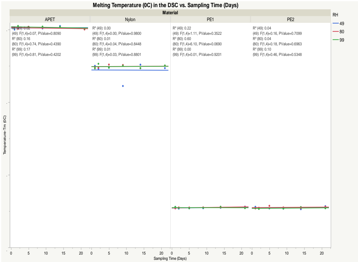
Figure 4.24: JMP Graph for Melting Temperature of ClO 2 Treated APET, Nylon-6, and PE (type 1, type 2) (°C) at 99, 80, and 49% Relative Humidities by Time (Days).
