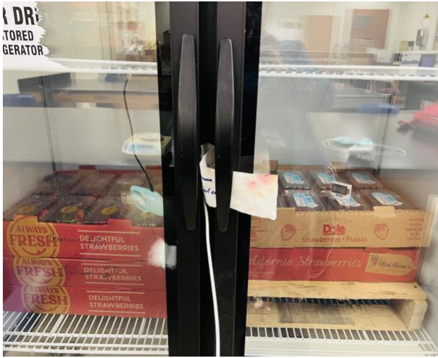
Figure 5.2.1 and 5.2.2: Experimental Apparatus – Pallet Strawberry Storage Exposed to a Slow Release of ClO 2 Gas Sachets (Low Dose, Continuous Release) at (60-70%) Humidity at (0 - 2 °C).
