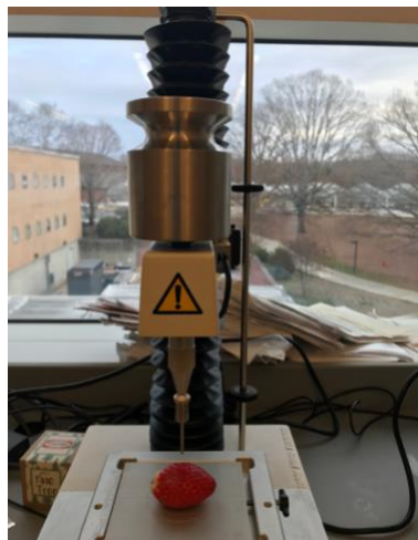
Figure 5.8: TA.TXPlus (Fruit Firmness Analyzer) for a Strawberry Sample
