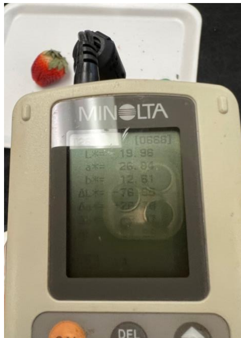
Figure 5.7: L^* , a^* , and b^* Values of a Strawberry Sample Using Minolta Colorimeter.
