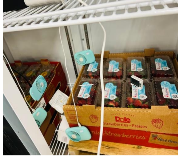
Figure 5.2.1 and 5.2.2: Experimental Apparatus – Pallet Strawberry Storage Exposed to a Slow Release of ClO 2 Gas Sachets (Low Dose, Continuous Release) at (60-70%) Humidity at (0 - 2 °C).
