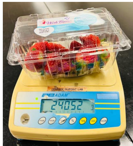
Figure 5.6: Weight Measuring of a Sample of Strawberry Clamshell Using an Analytical Balance.
