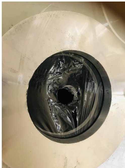
Figure A-1: Dart Drop Impact Tester (ASTM D4272M-15)/ISO7765-2).
