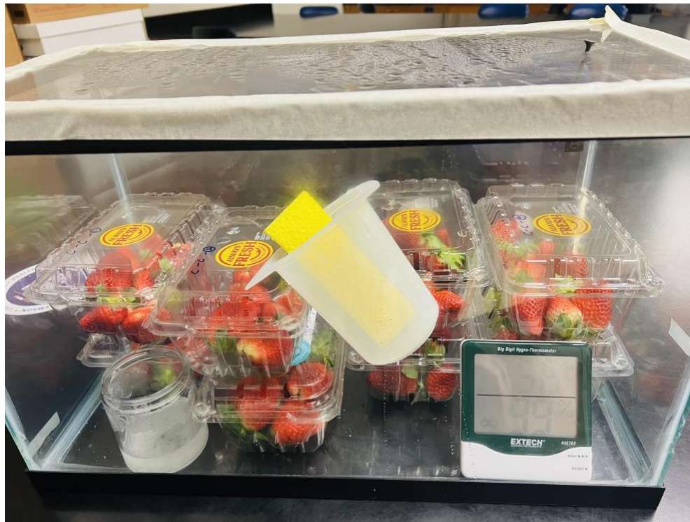
Figure 5.3: Experimental Apparatus – Chamber Strawberry Storage exposed to slow release of \text{ClO}_2 gas sachets (low dose long time of release) at (99%) humidity at (0 - 2 °C).
