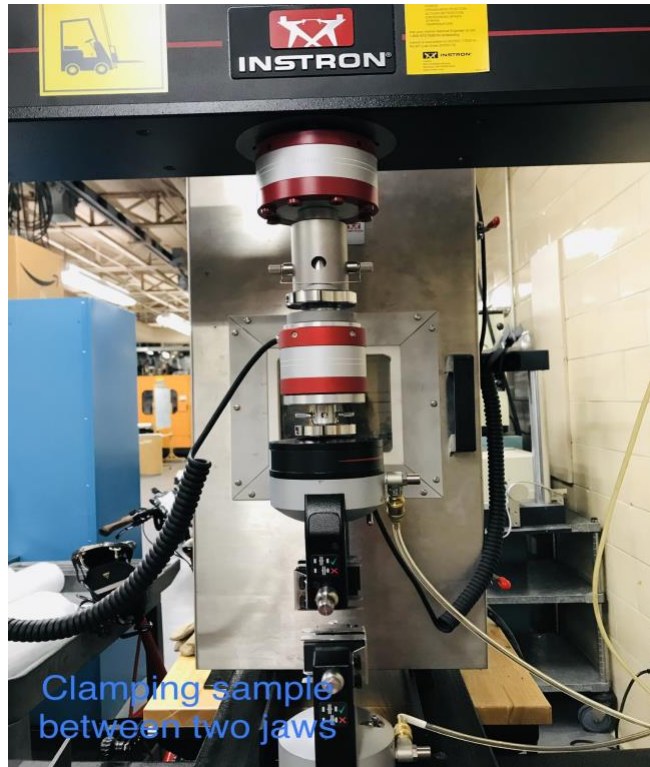
Figure B-1: Example of Nylon Film Clamped Between Two Jaws of Tensile Tester (Instron).
