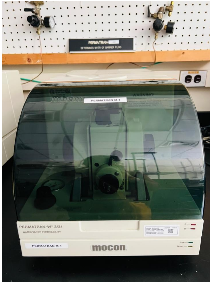
Figure C.1: MOCON PERMATRAN-W 3/31, Module M-1 That Measured Water Vapor Permeability of Packaging Materials.
