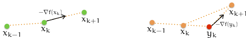
Figure 1.2: A typical iteration of PGD (on the left) and a NAGD iterate (on the right). Image is from [47].
