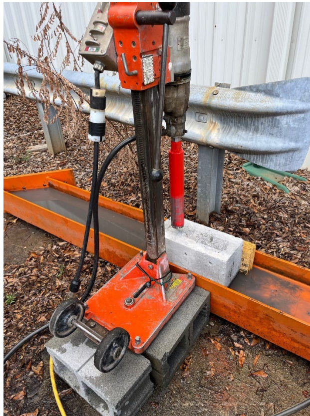
Figure 20. Coring Drill Setup
