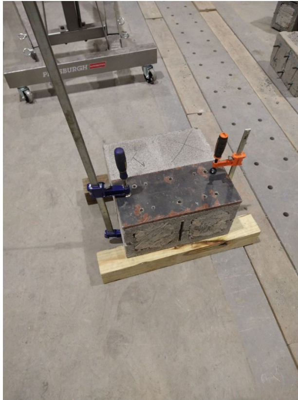
Figure 22. Steel Plates Clamped to C1072 Specimen
