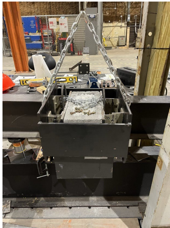
Figure 7. Member 6 being put into place using crane and angles
