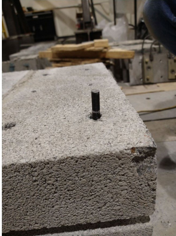
Figure 25. Threaded Rod in Drilled Hole
