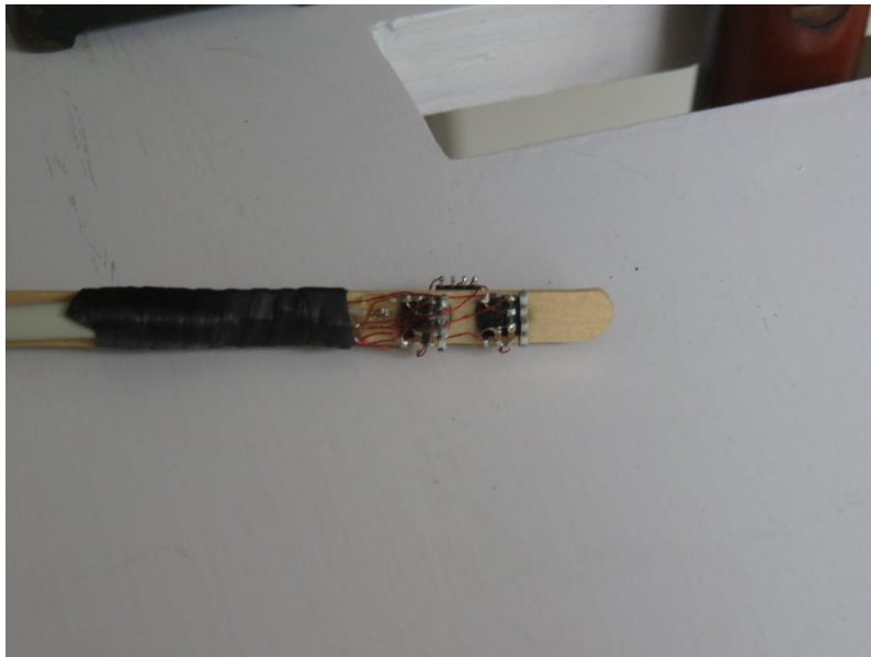
Figure D2: Magnetic sensors and amplifier attached on both sides of a wood stick
