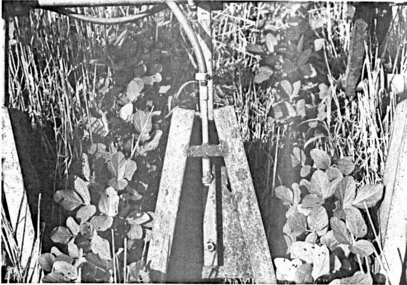
Figure 7. The experimental prototype directed-spray applicator was outfitted with 80-degree flat fan nozzle tips enclosed in an A-shaped framework constructed specifically for 20-inch rows.
