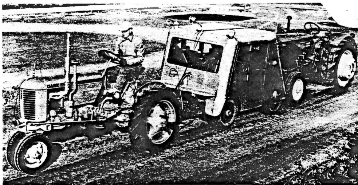
Figure 2. A Nebraska test car and tractor (Case VAC) being tested in 1949. The Nebraska tests have become a standard for the United States and for many foreign countries. The tests have been responsible for the removal from the market of many tractors of inferior design (Gray, 1954).
