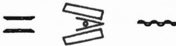
Figure 2. Schematic of soil engaging components on the John Deere Model 7100 Max-Emerge planter.
