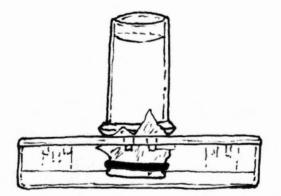
Fig. IV-3. Inverted vial is positioned with nylon screen below level of water and above base of tray.
