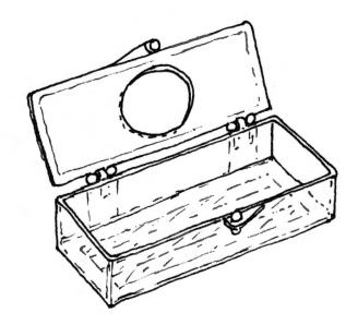
Fig. IV-2. Plastic counting tray with grid. Opening in lid was made with a heated pipe and allows vial to be suspended in tray.
