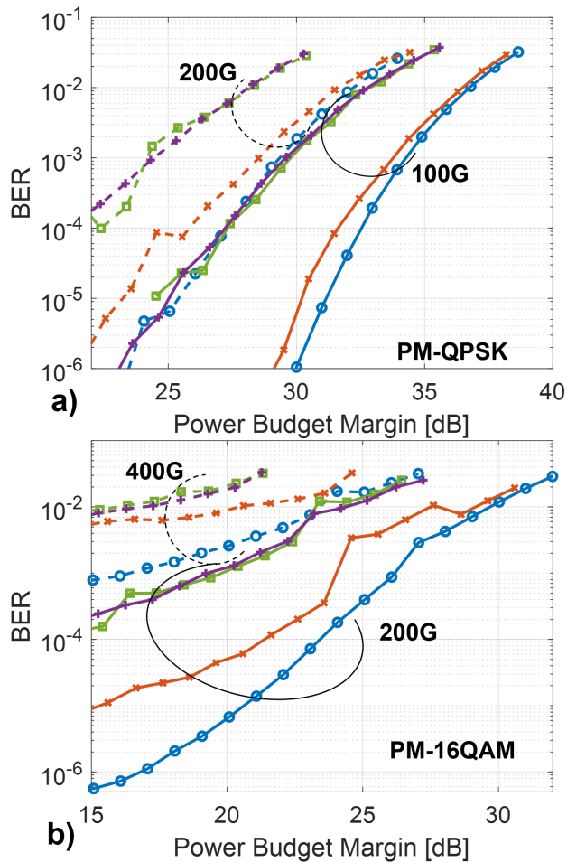
Fig. 4. Measured BER vs power budget margin for a) PM-QPSK and b) PM-16QAM modulation in different conditions: back-to-back (blue, circles), 'OM3 only' (red, crosses), '3 \mu\text{m} offset-3 \mu\text{m} offset-OM3' (green, squares) and '3 \mu\text{m} offset-OM3-3 \mu\text{m} offset' (purple, plus signs) configurations.
