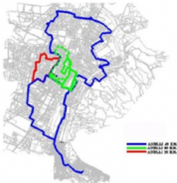
Fig. 1. Turin deployed urban fiber infrastructure exploited for the experimental assessment of the proposed sensing solutions.
