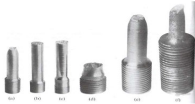
Figure 5 - Some Types of Fractures - (a) “cup-cone” type; (b) Fragile; (c) Mixed; (d) Fragile; (e) Rosette; (f) Shear.
