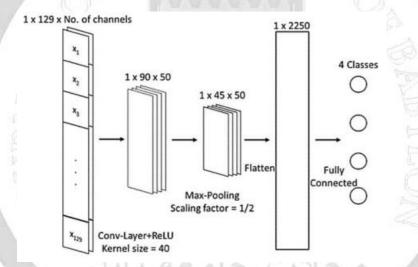
Figure 3: Architecture of Convolutional neural network
