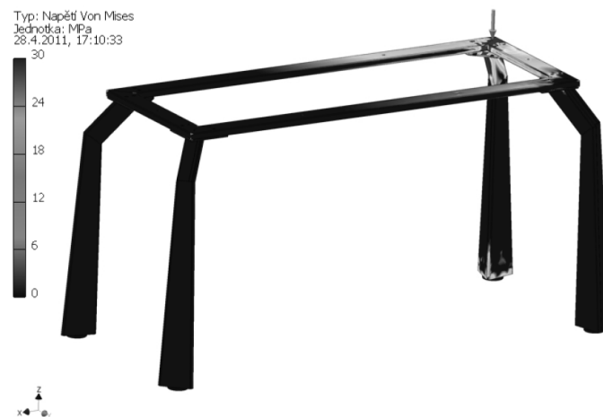
Figure 5: Equivalent tension (von Mises) when the apron is loaded in the corner.
