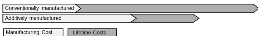
Figure 8: Comparison of total costs of the bracket including manufacturing and lifetime costs.
