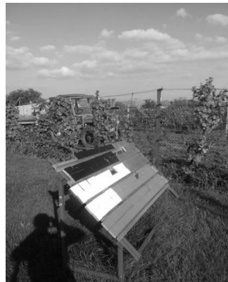
Figure 2: Outdoor exposition of the tested samples in South Moravia.
