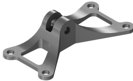
Figure 2: Damping bracket of an aircraft by milling [8].
