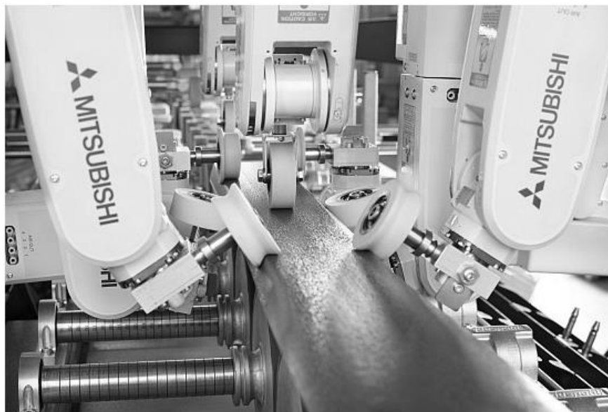
Figure 5: Automatically set profile-wrapping machine “RoboWrap” [9].
