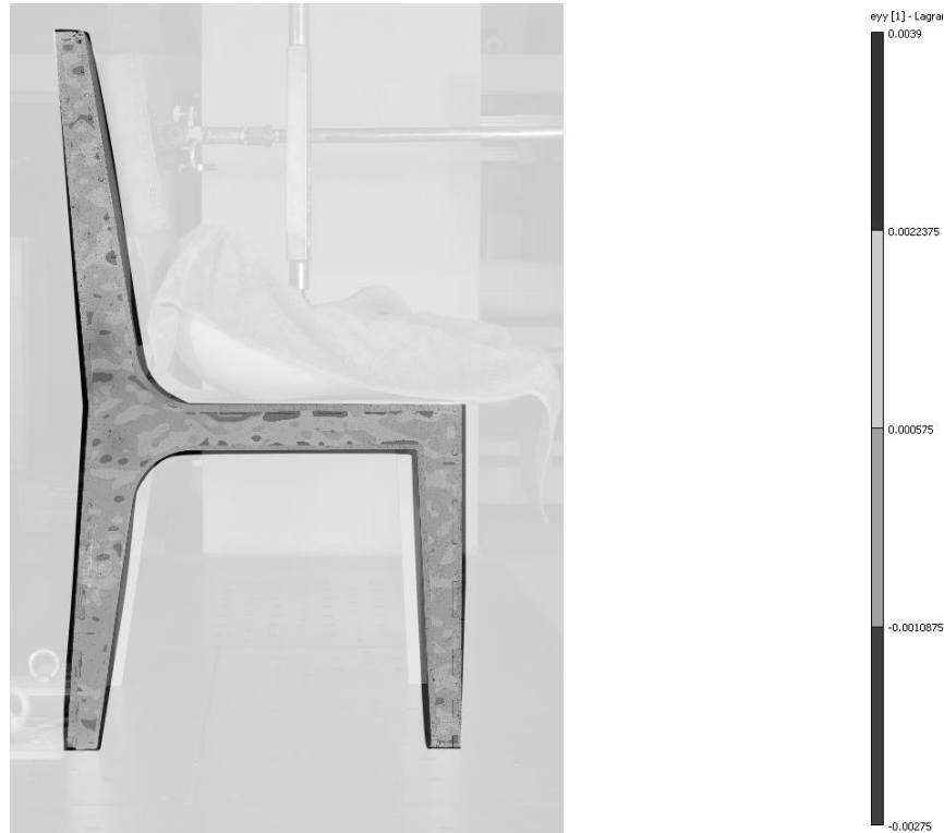
Figure 3: The strain field in vertical direction ( \epsilon_{yy} ).
