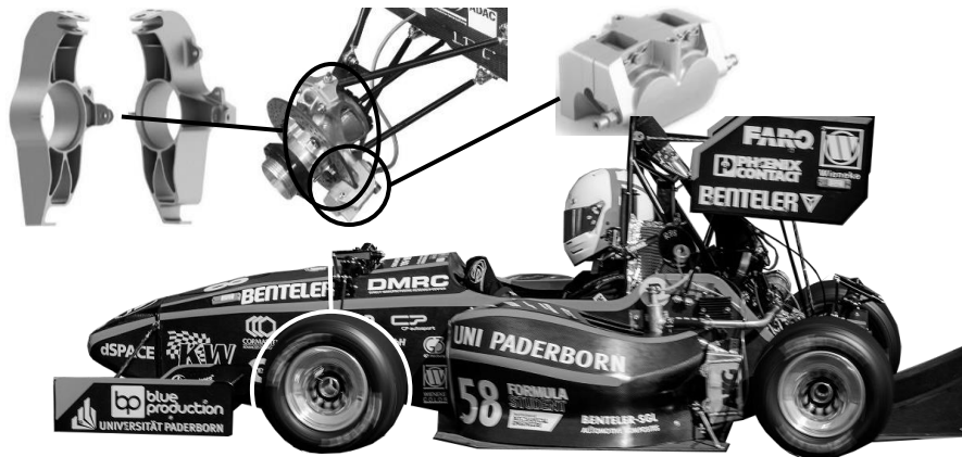
Figure 1: Formula Student car from UPBracing Team with enlarged suspension and sample part upright (left) and brake caliper (right).
