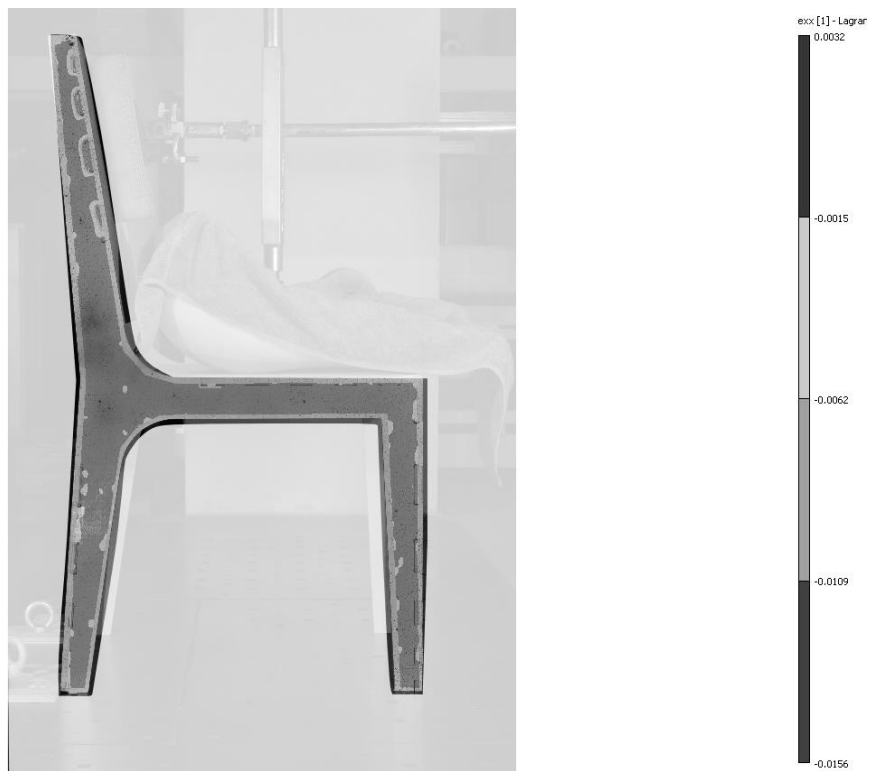
Figure 2: The strain field in horizontal direction ( \epsilon_{xx} ).
