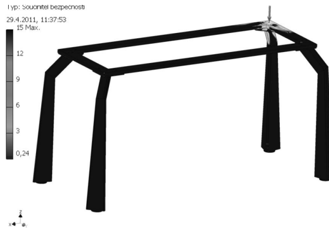
Figure 6: Coefficient of safety when the apron is loaded in the corner.
