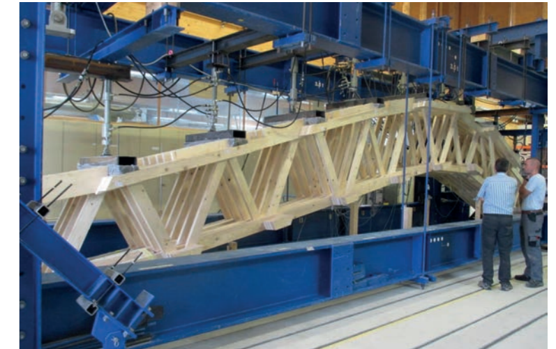
Fig. 11: Execution of support tests
