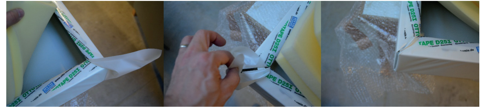
Fig. 10: Detail of corner solution for the foil wrapping. The foil is drawn inwards through the open corner.
