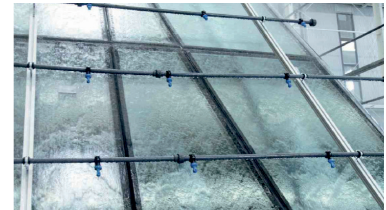
Fig. 8: A physical mockup is tested acc. to driving rain in the laboratory (Schüco International KG, 2017)
