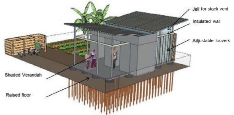
Fig. 8: Climate resilient affordable housing unit proposed for Chennai city (Courtesy: Biome Environmental Solutions)
