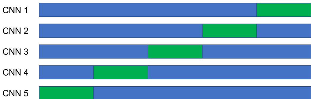
5 Schematic representation of the cross-validated approach in training the individual neural networks, training data in blue, validation data in green
