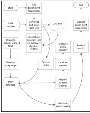
Fig.3: Experiment flow for proxy evaluation
