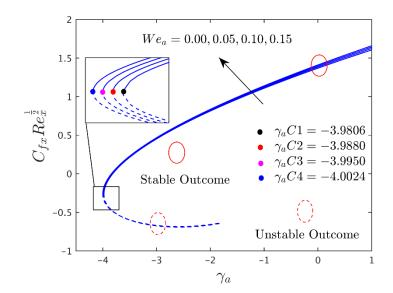
**Figure 5.** Influence of *We*<sup>*a*</sup> on axial shear stress.
