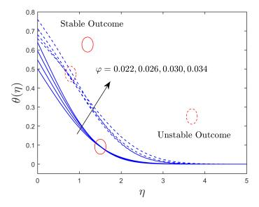
**Figure 12.** Influence of  $\varphi$  on the temperature profile.
