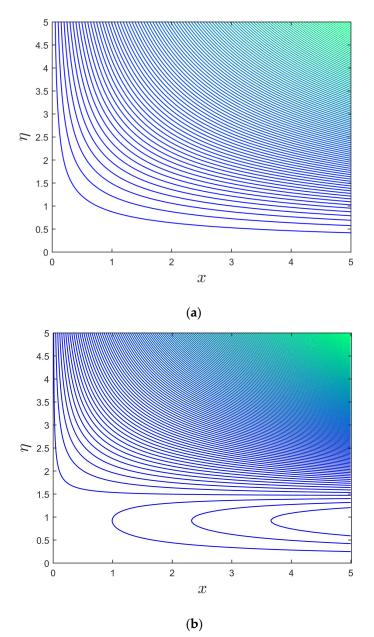
**Figure 13.** (**a**,**b**): Streamline profile for the branch of upper and lower solutions when m = 0.0.
