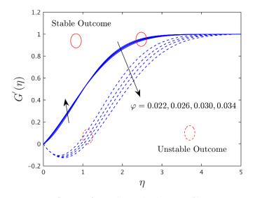
**Figure 10.** Influence of  $\varphi$  on the axial velocity profile.
