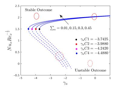
**Figure 4.** Influence of  $\Sigma_a$  on heat transfer.
