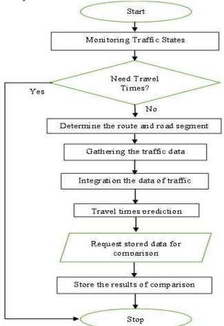
Figure 1. The flowchart for main predict travel times of vehicle
