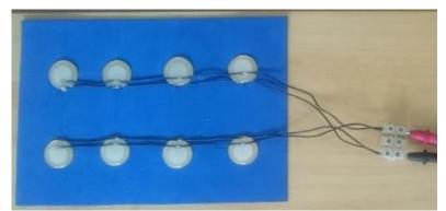
Figure 4. Tile with piezoelectric discs connected in parallel
