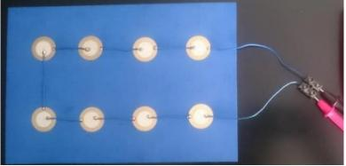
Figure 3. Tile with piezoelectric discs connected in series
