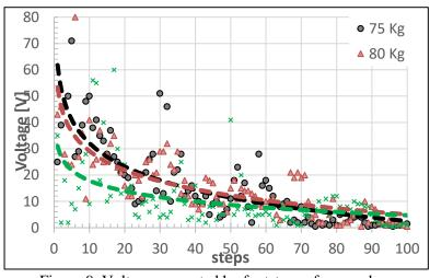
Figure 9. Voltage generated by footsteps of passersby
