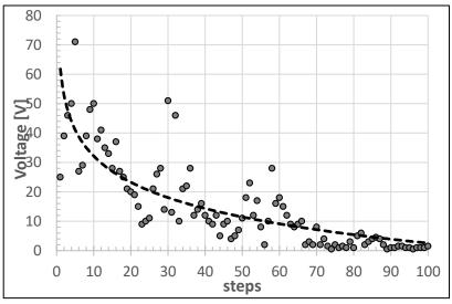
Figure 6. Voltage generated by the steps of a 75 Kg person
