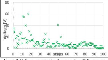
Figure 8. Voltage generated by the steps of an 85 Kg person
