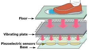
Figure 1. Flooring Tiles with Piezoelectric Crystals [22]
