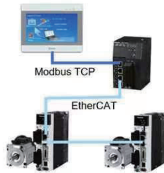
Figure 2. Topology scheme of controller system
