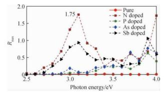
Figure 3. Photoresponse of intrinsic and doped monolayer WS2<sup>[4]</sup>.
