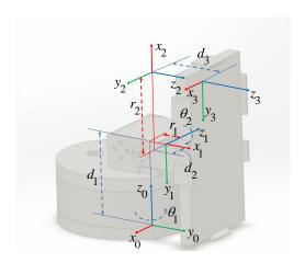
Figure 3. Manipulator kinematics coordinate system
