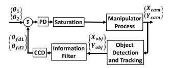
Figure 5. Visual Object Tracking Control Block Diagram
