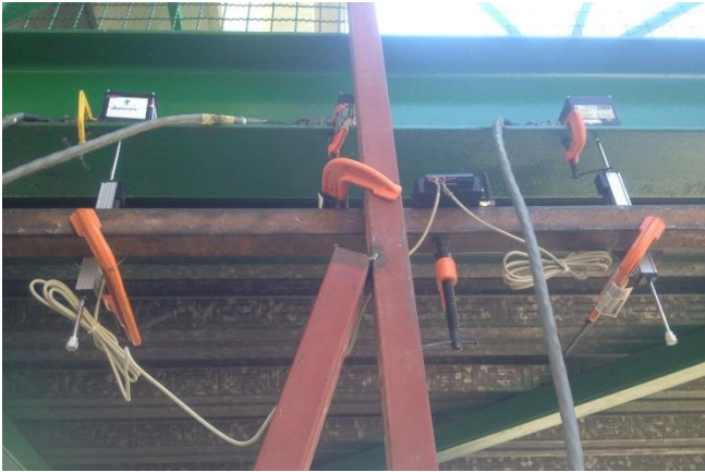
Fig. 5. Instrumentation setup of the pedestrian bridge.
