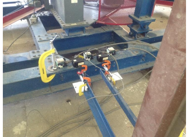
Fig. 2. Instrumentation setup for the quasi-harmonics tests.
