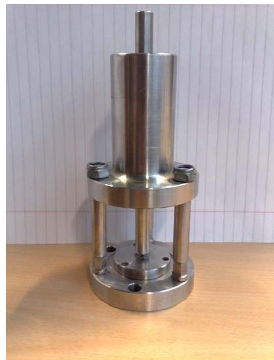
Fig. 2 Assembled ASTM F 394 test jig, no specimen installed
