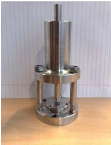
Fig. 1 Bi-axial flexural strength test jig
