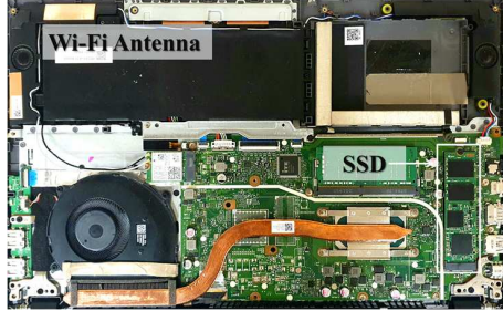
Fig. 1. A picture of the device under test with the target SSD.
