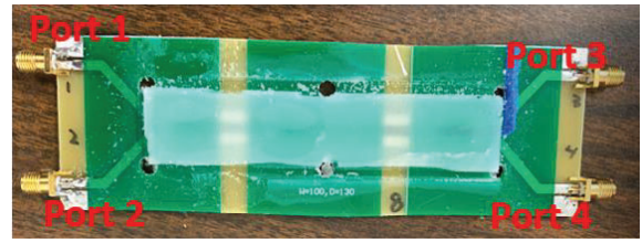
Fig. 3. Microstrip traces covered with the coating material.
