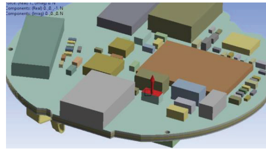
Fig. 7. External force is added on the MLCC as shown with the red arrow.
