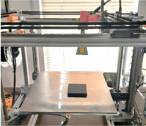
Fig. 8. Setup of the SAR reflectivity scan of the designed absorber.
