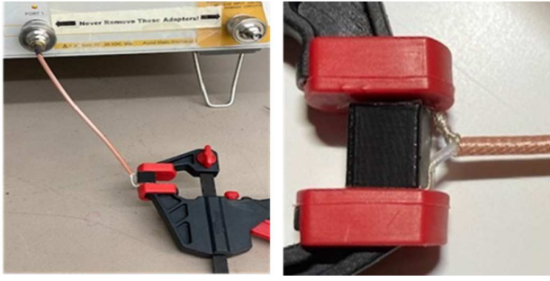
Fig. 1. (Left) An image of the parallel plate capacitor connected to the VNA via a coaxial cable and mechanical clamping. (Right) An image of the mechanical clamping used in this measurement. The red blocks are the jaws of the clamp, the black cube is the printed CF20 sample, and the silver wires are the center conductor and shield of the coaxial cable used to connect the parallel plate capacitor to the VNA for measurement.
