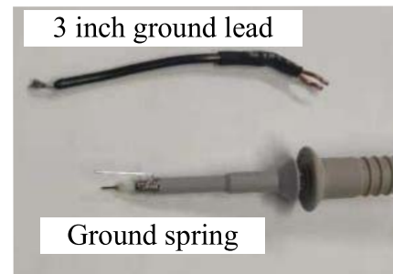
Fig. 21. Photograph of different grounding structures.
