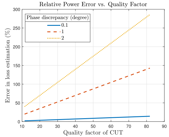
Fig. 2. Error versus Q factor for different phase discrepancy levels.
