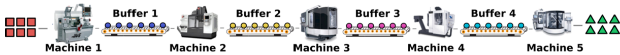
Fig. 2. A typical manufacturing system with N machines and N - 1 buffers (here N = 5 ).
