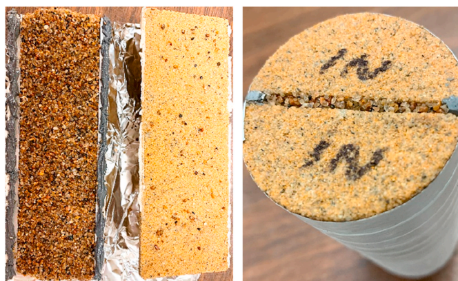
Fig. 2. Photo of sandwich-like channel model. The model consisted of two semi-cylindrical cores (mimicking reservoir matrices) and a sand-filled high-permeability channel between the cores.
