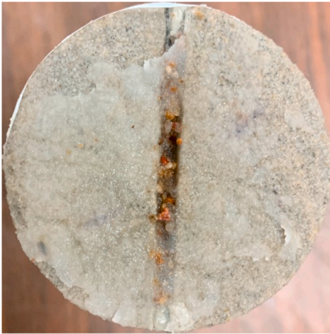
Fig. 10. A gel cake formed at the inlet surface of a channel model (Exp #19, 139 darcies, particle/pore ratio = 1.27, matrices 167 md). [Due to the high threshold pressure at the inlet surface of the matrices, a cake formed and further prevented the gels from invading the matrices. On the other hand, the low threshold pressure in the channel (5.0 psi) allowed easy penetration of the gels into the channel. As a result, the microgels selectively penetrated and placed in the super-k channel. After the gel treatment, the cake could be removed by soaking with chemical breakers to resume the injectivity of in the matrices. Selective penetration behavior was also observed in microgel treatment experiments in polymer flooding (Zhao et al., 2021b).].
