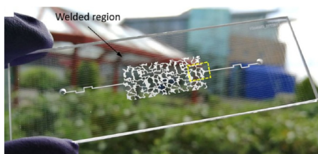
Figure 12. Glass model by laser engraving. Reproduced with permission from ref 27. Copyright 2019 Springer Nature.
