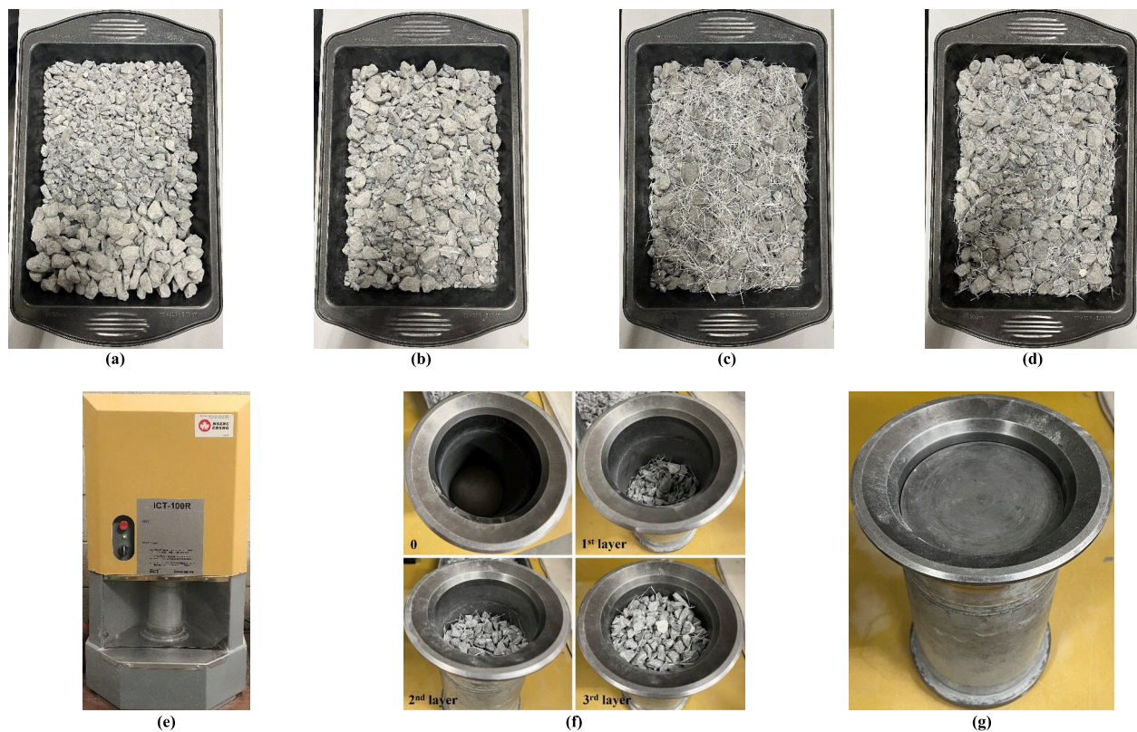
Fig. 2. Procedure of PD measurements, including (a) weighing different coarse aggregate classes, (b) homogenizing coarse aggregate, (c) adding fibers to coarse aggregate, (d) homogenizing F-A mixture, (e) ICT set-up, (f) layer-by-layer filling of cylindrical specimen, and (g) flattening the specimen's top surface.
