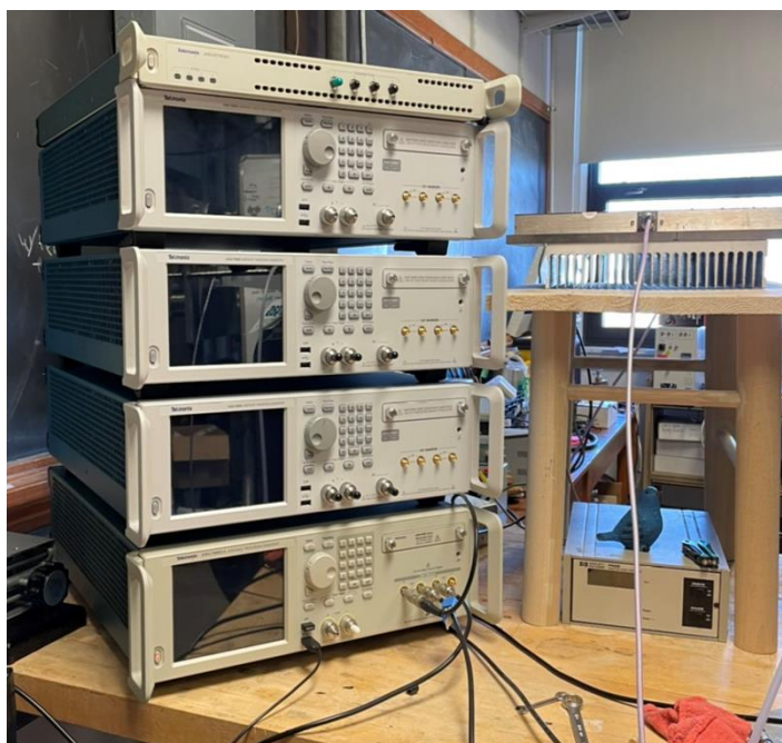
Figure 2. Picture of the Tektronix® AWG 70000 AWGs (bottom) with the Tektronix® AWG SYNC01 synchronization hub (top). The synchronization hub works on up to four AWGs at one time.
