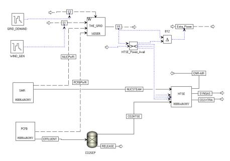
**Figure 7.** Coal–wind–nuclear hybrid energy system to produce low-carbon electric power plus chemicals or fuels [22].
