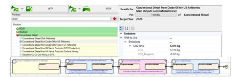
Figure 5. LCA results for conventional diesel produced from crude oil.
