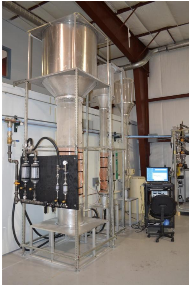
Figure 3. Photo of the two fluidized beds set-up along with the air flow system used in this work.
