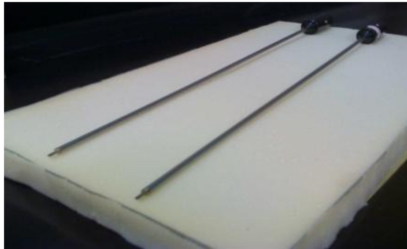
Figure 4. Optical Probe (PV6) System (Institute of Process Engineering of the Chinese Academy of Sciences).
