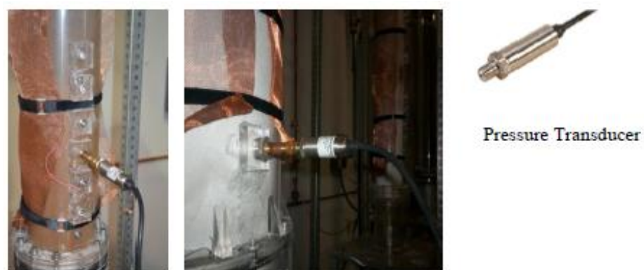
Figure 10. Pressure transducer being mounted on the 0.14 m and 0.44 m inner diameter fluidized beds.
