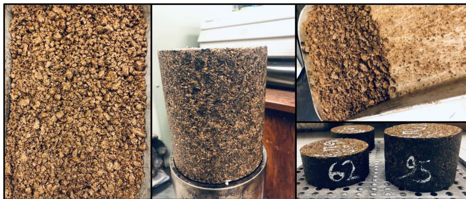
Fig. 3. Neat guayule mixture (G-Mix): loose and compacted.
