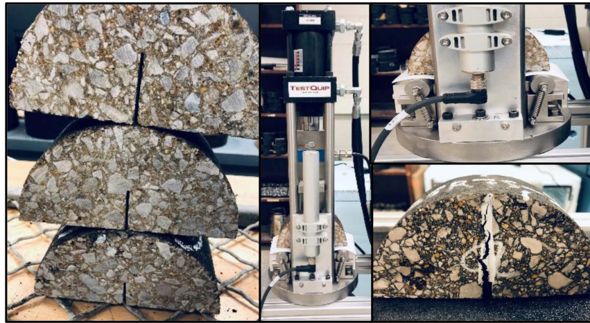
Fig. 7. Technical steps from the SCB test procedures.
