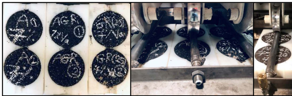
Fig. 5. Technical steps from the rut test procedures.
