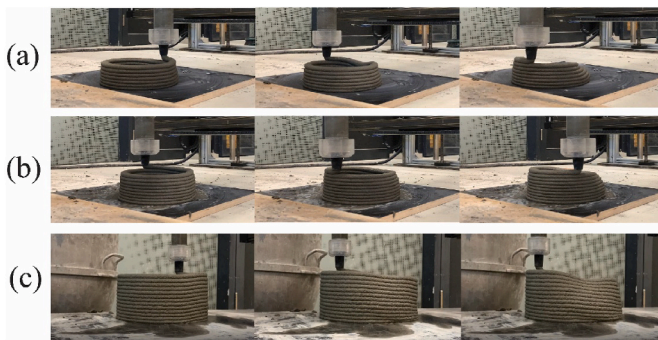
Fig. 9. Snapshot of the plastic collapse failures occurred during the printing trials at print speed of 80 mm/s (a) NC1-F0 (b) NC1-F1 (c) NC1-F2.
