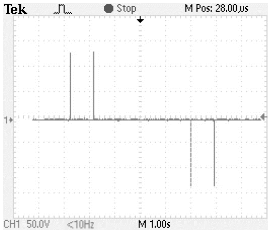
Fig. 5 Waveforms generated using the electro stimulator with a 1kΩ connected at the output.
