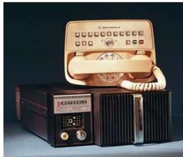
Figura 2.7: Mobile Telephone Service (IMTS)
