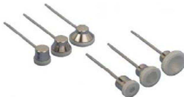
Figure 2. The six different models of the Leipzig applicators: cone shaped, 92% tungsten and 8% steel alloy devices, with apertures of 1, 2 and 3 cm. Three are for horizontal source loading and three for vertical source loading.
