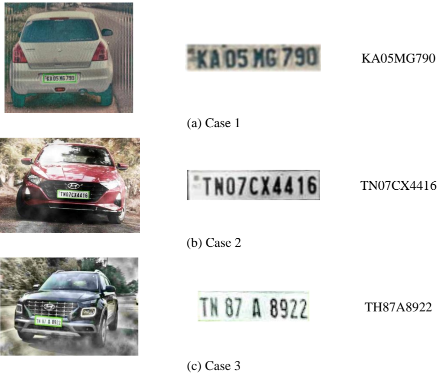
Fig. 10 Preprocessed images and corresponding recognition of vehicle's number plates
