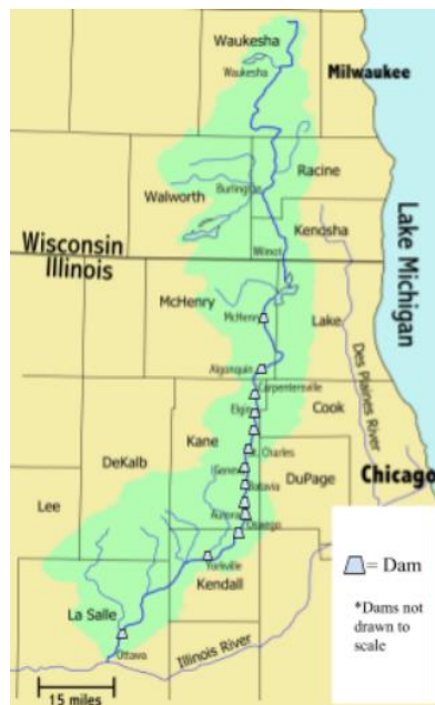
Figure 24 Locations of dams currently along the Fox River between McHenry and Dayton, Illinois.
