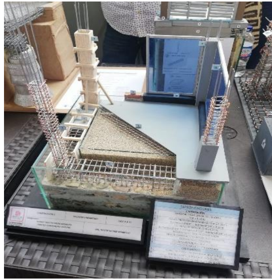
Figure 2. Construction process of a porticoed system.
